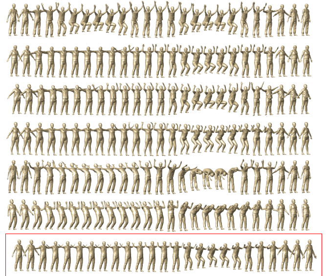
Figure 10. Example of a mean 4D surface (highlighted in red) computed on six 4D surfaces from the CAPE dataset after their spatiotemporal registration. The input 4D surfaces perform different actions: the 4D surfaces in the first four rows perform a squat action while the last two perform a back and forward bending action; see the Supplementary Material for additional results.
